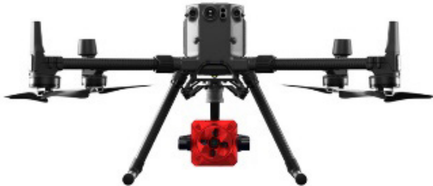
Figure 6 Combination: Matrice 300 RTK and Zenmuse L1 + Zenmuse P1.
